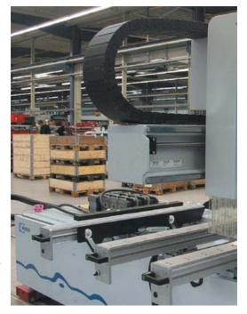
There is little space available and the cables are extremely stressed due to complex movements. Feed rates are at 328 ft/min and the travel length at 13 to 20 ft. Drilling speed is 24,000 revolutions. The cable carriers had to be quick to install and maintenance-free. In addition, it had to be able to withstand chips and dust. For this reason, the cable carriers are supplied as completely enclosed energy tubes, which are completely immune to flying debris and woodchips.
